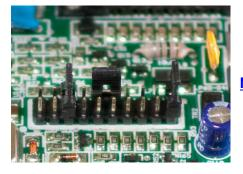
**NOTE:** the CAT interface is **not configured** at the factory. Jumpers are shown configured for RS232 levels.
